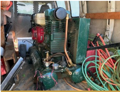
Gas-powered air compressor that was used to power nail guns.
