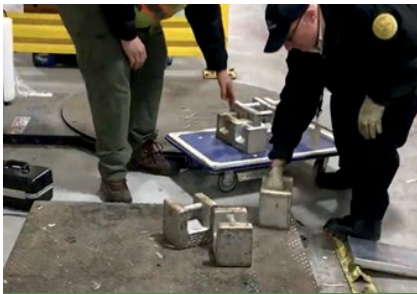
Employees manually transferring 50 lb. standard weights onto large floor scales
