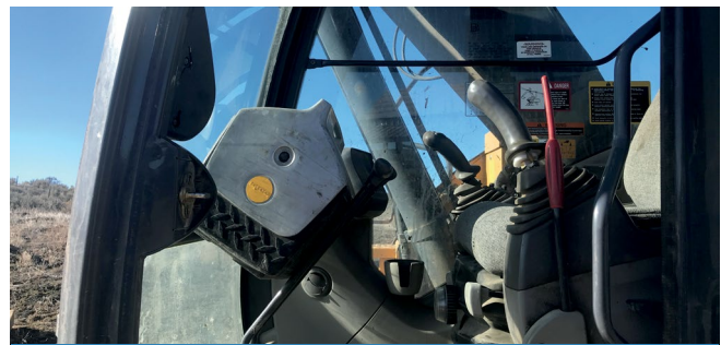
The lunch box the excavator operator stowed between the windshield and the directional controls of the excavator
