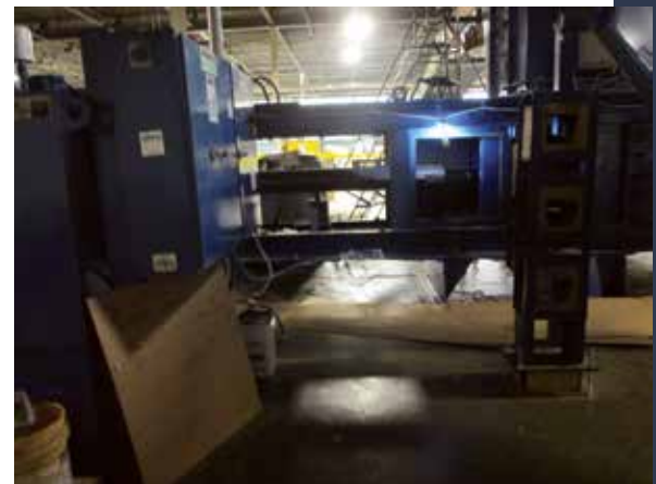
International Press and Shear horizontal auto-tie baler and unguarded opening. The right opening is where it was unguarded. The blue metal device to the right of the opening slides with the shaft. The employee's head was in the opening when the baler was activated, causing the employee to be decapitated.
