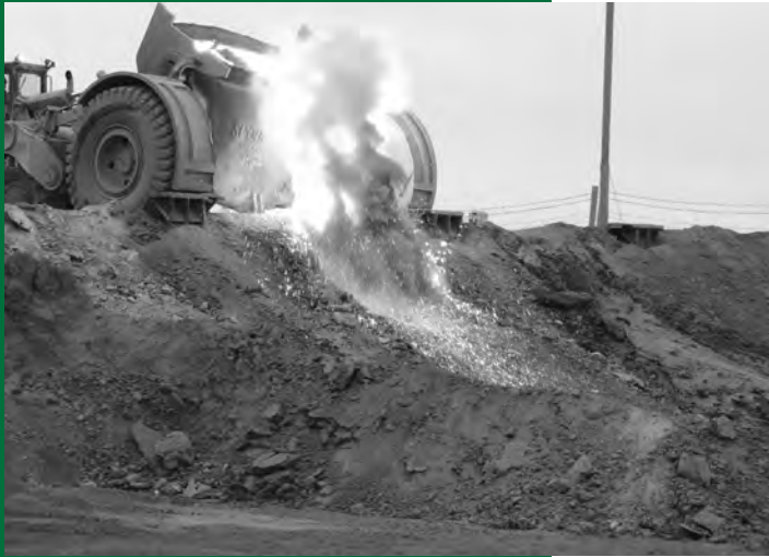
An employee dumps approximately 50 tons of hot slag into a designated cooling area.
